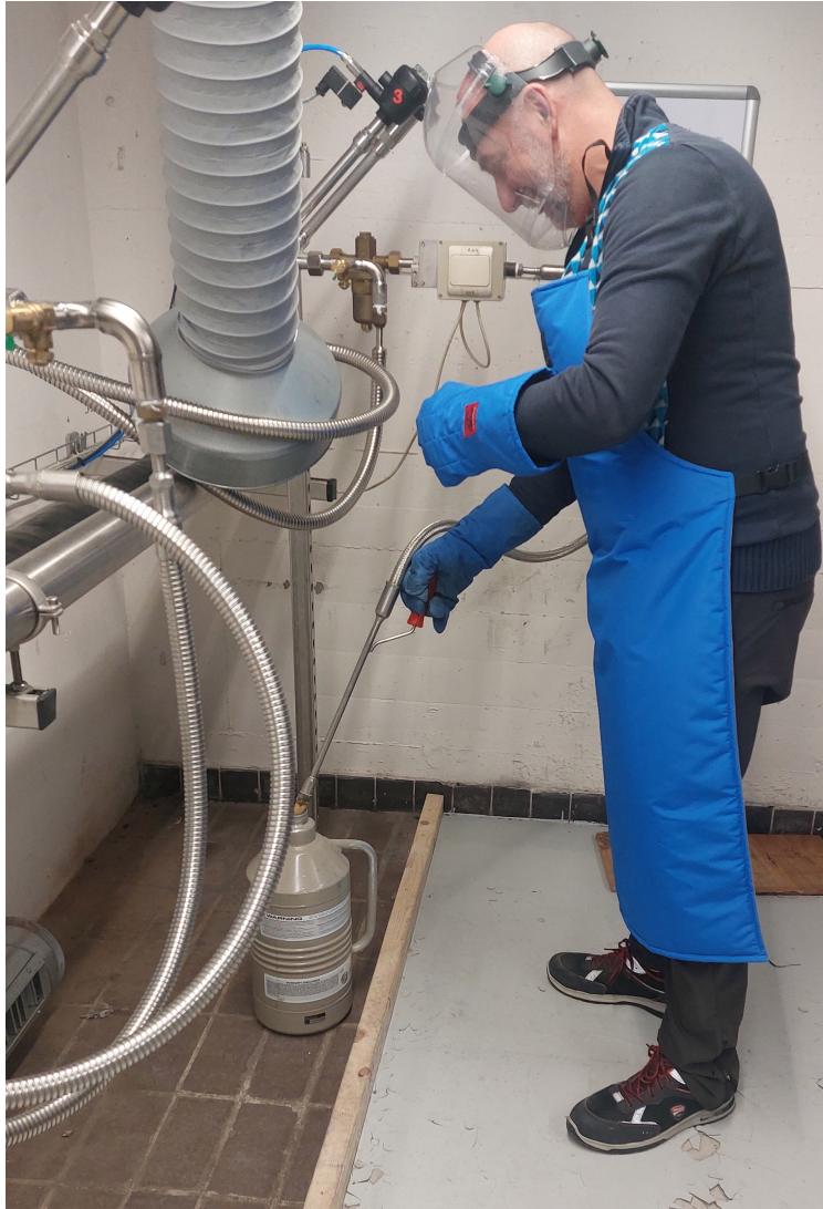
Figure 6: Proper working methods with cryogenic substances require, among other things, the correct clothing.
