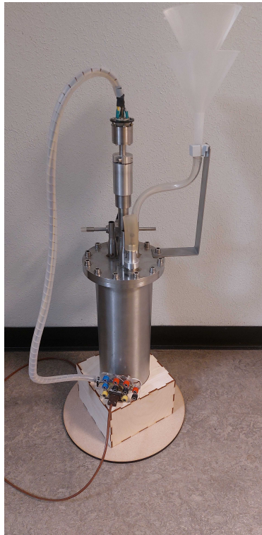
Figure 33: The cryostat with electronics.
