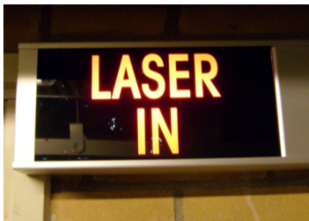
Figure 15: Warning lights above the doors indicate whether the laser in the room is in use.
